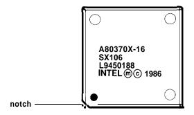
Align the notched corner of the coprocessor with the notched corner of its socket. The notched sides must be aligned for the coprocessor to operate properly, so be sure its position is correct before you go to the next step.
